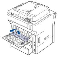
7. While pushing the fuser lever to the right, open the fuser door.
